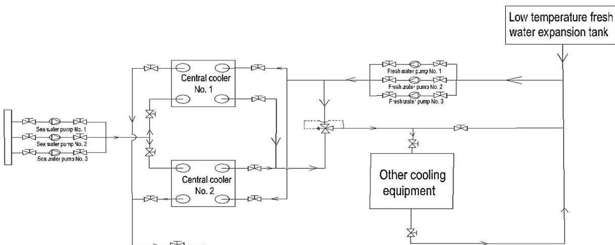
Figure 2. Frequency conversion sea water pump cooling system
